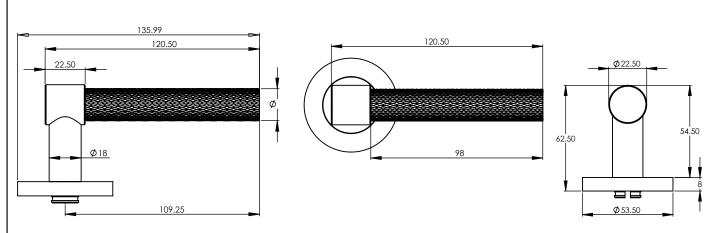
This latch handle is suitable for use with most U.K. tubular latches.
