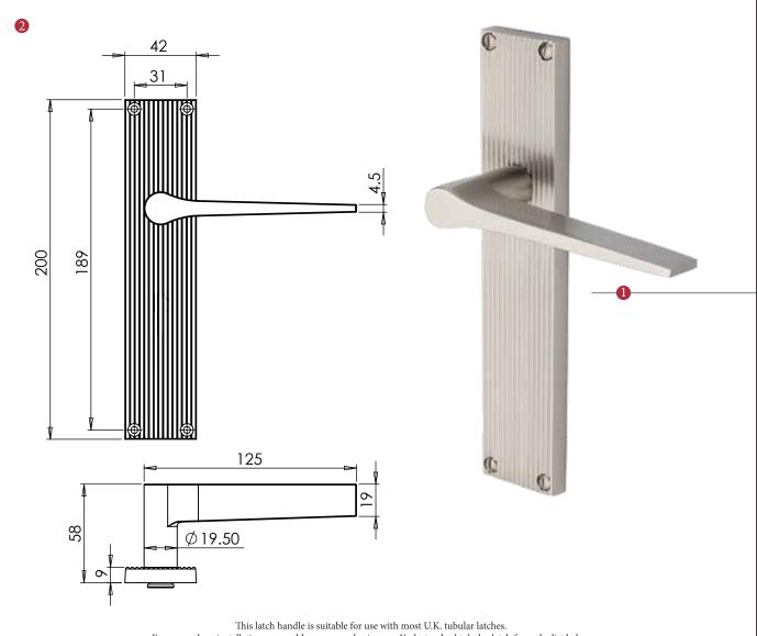
For a new door installation we would recommend using our York standard tubular latch from the list below.
